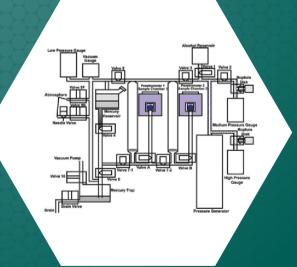
The cell is closed with a lid and placed in the sample chamber. Intrusion volume of mercury is measured by noting changes in mercury level in the penetrometer with a magnetic sensor. Exposure to mercury is negligible due to the unique design of the instrument. The unique design also permits use of nonmercury nonwetting liquids for intrusion. Another instrument design uses water as the nonwetting liquid and uses absolutely no mercury. The instrument is known as the Aquapore.
