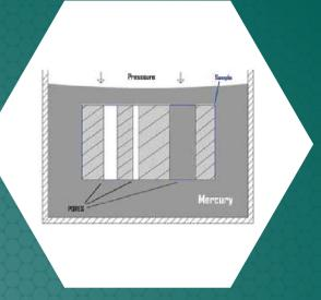
the volume of intruded nonwetting liquid are accurately measured. Combining these data with the surface tension and the contact angle of the liquid, pore diameter, pore volume, pore volume distribution and pore surface area are computed.
